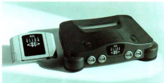
The finished Ultra 64 unit has a matt-black casing, features four joypad ports and uses a cartridge format similar to that of the SNES
